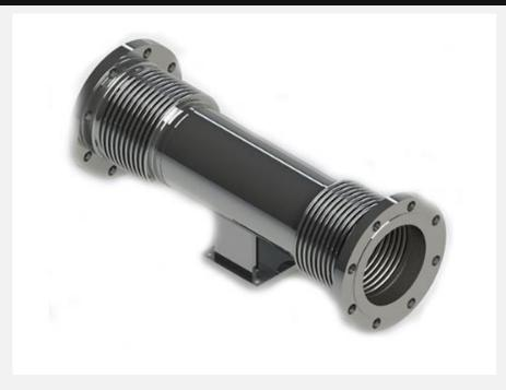
A double gimbal expansion joint consists of two single gimbal expansion joints connected by an intermediate pipe. This configuration allows for the absorption of significant lateral movement in any plane at each end of the joint.
